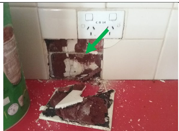
Photo 7: No asbestos detected in sample 6-270721. Ceramic tile adhesive of splash back in Kitchen/Dining.
